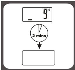
Auto shut-off occurs if display shows '0' or shows the same weight reading for 2 minutes.
