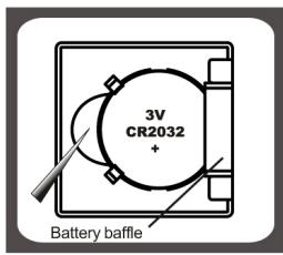
Open the battery compartment cover at the back of the handle.
